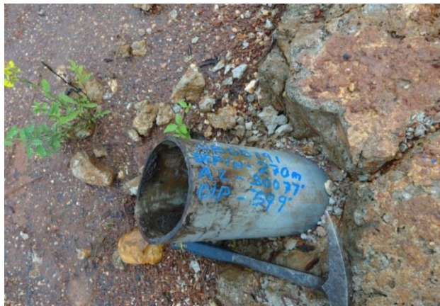
Figure 11: preserved drill hole collar PVC pipe
