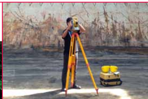
Az United staff performing volumetric survey of sand
