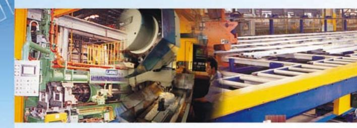
state-of-the-art material handling system from the USA complete with double pullers, an automatic stretcher and a cutting saw as well as a US made billet heater with a log shear.
