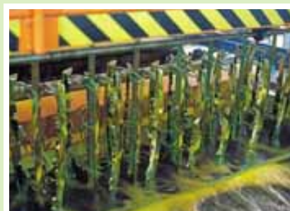
Plastic parts undergoing Chrome Plating process
