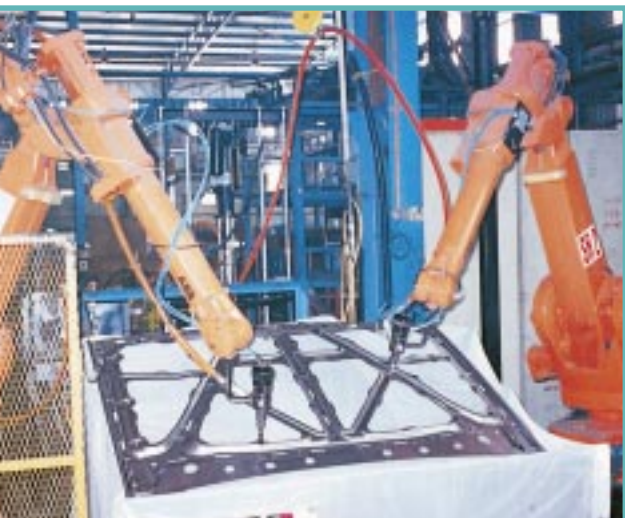
A pair of Robotic Arms for application of sealant
