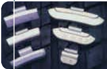
A variety of TRAX tin weights. Plastic coated tin weights are recommended for alloy wheels to minimise electro-chemical corrosion.
