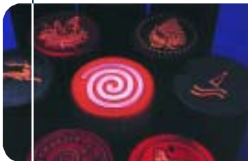
A variety of TRAX tin weights. Plastic coated tin weights are recommended for alloy wheels to minimise electro-chemical corrosion.
