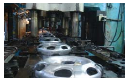
Press Operations – Progressive stamping of discs for domestic and regional exports
