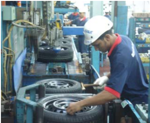
Balancing Operations – Key process in tyre assembly operations to assure Noise, Vibration and Harshness (NVH)
