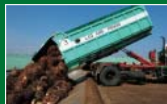
FFB unloading direct from truck onto ramp
