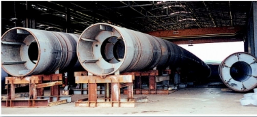
Fabrication and Fit-up of Arch segments for Bridge BR-8 at Putrajaya
