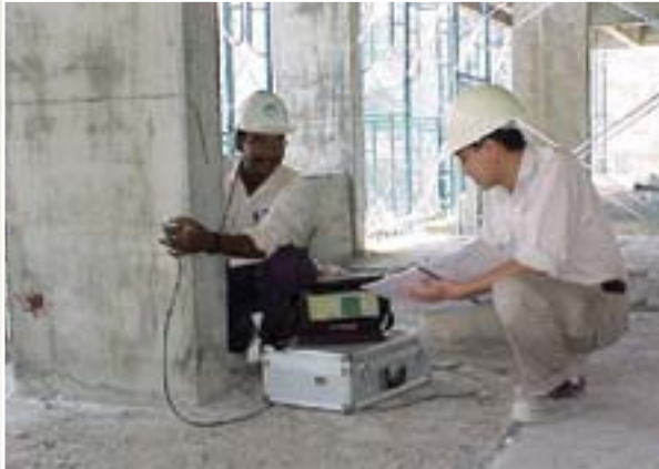
Meter testing of concrete cover
