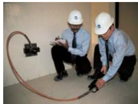
Pull-off test for internal wall tile
