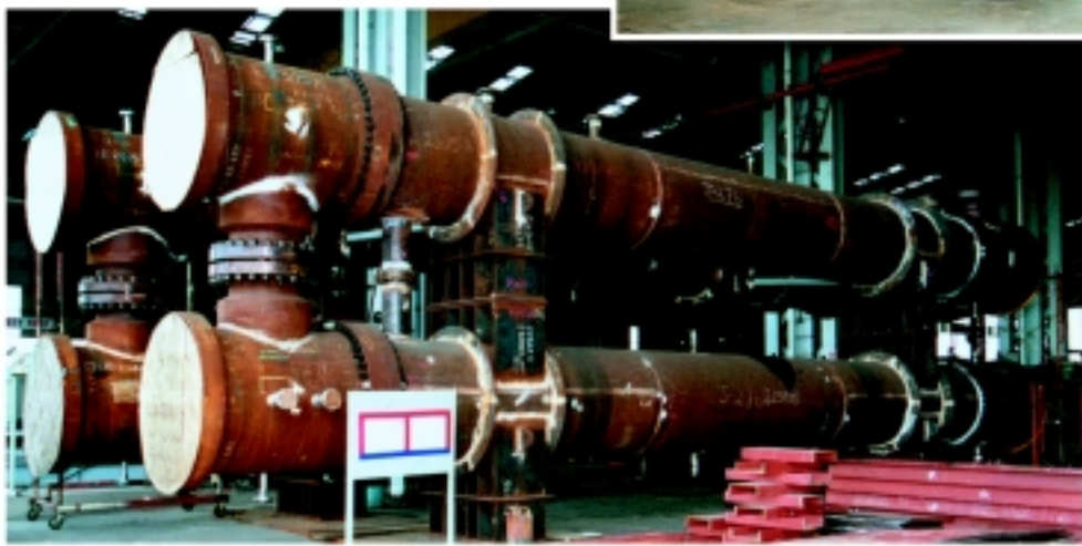
Fabrication of Shell and Tube Heat Exchangers at Torsco's Lumut Plant No.2 for CTOC Cakerawala, a Malaysian-Thai joint-development project in South China Sea
