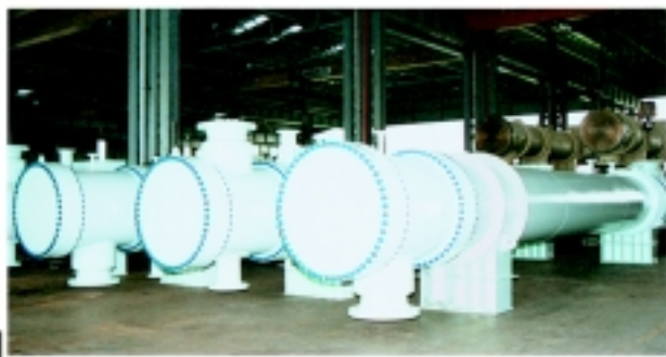
Fabrication of Shell and Tube Heat Exchangers at Torsco's Lumut Plant No.2 for CTOC Cakerawala, a Malaysian-Thai joint-development project in South China Sea
