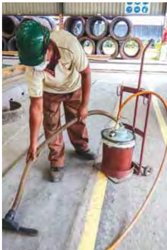
Pneumatic vacuum cleaner is effective in cleaning up dust in ICP factories
