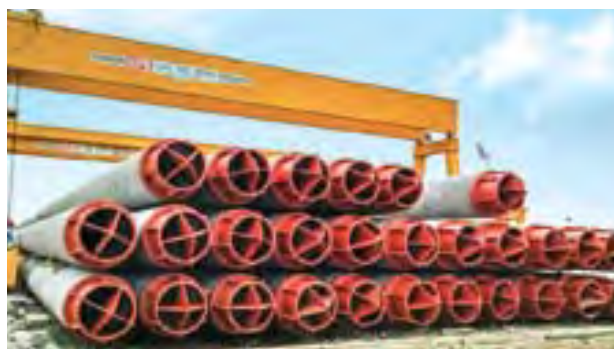
ICP Piles with special shoes for the New Deep Water Terminal, Kuantan Port, Pahang
