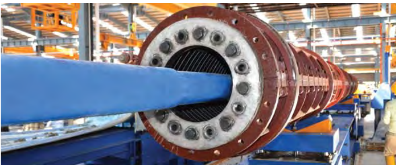
Concrete feeding process of ICP Piles using concrete pumping technology
