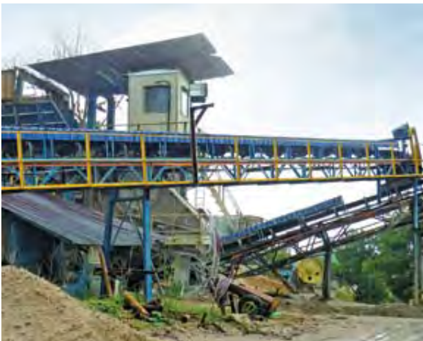
Covered conveyor - Dust control measure at MRP Kulai
