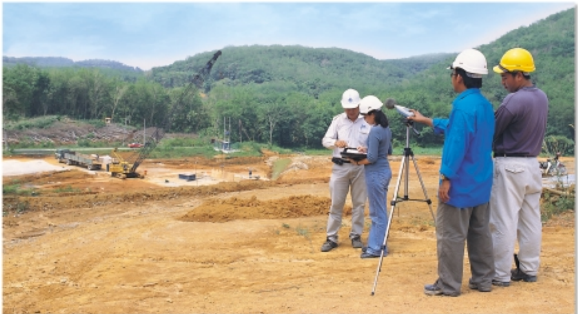
Measurement of noise level generated by construction machineries at an open space within the nearest residential area of Jalan Lingkaran Bandar U4 project in Putrajaya
