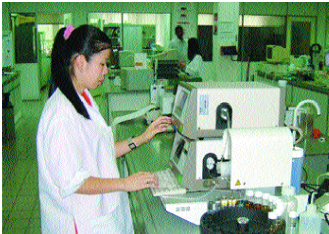
Testing our product for original gravity, alcohol and extract
