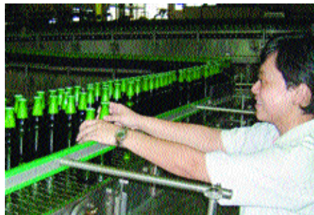
Taking a sample from the bottling line for a quality check
