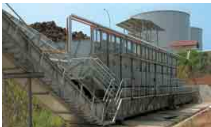
Oil Mill front-end upgrading incorporating the use of continuous chain transfer technique that improves FFB handling and logistics at Diamond Jubilee Oil Mill.
