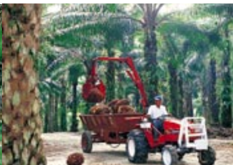
Infield mechanisation – FFB collection using a grabber.
