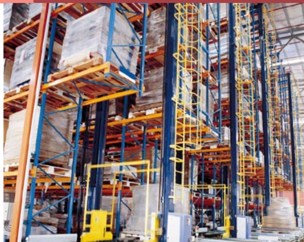
The state-of-the-art Automatic Storage and Retrieval System available at the Genting Sanyen box plants.
