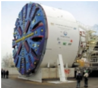
Tunnel-boring machine (TBM).
