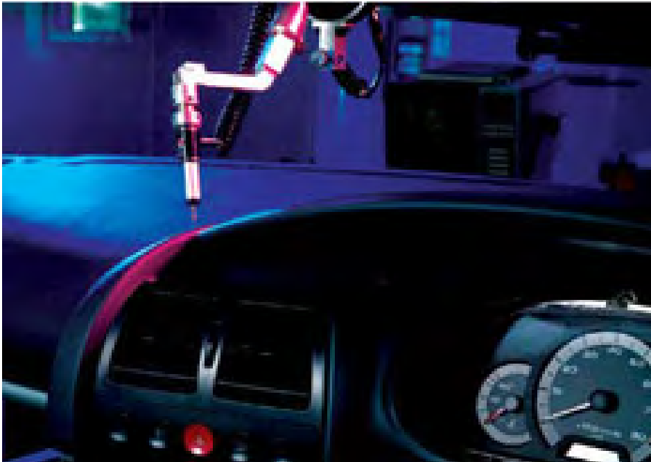
Coordinate measurement of Instrument Panel Assembly
