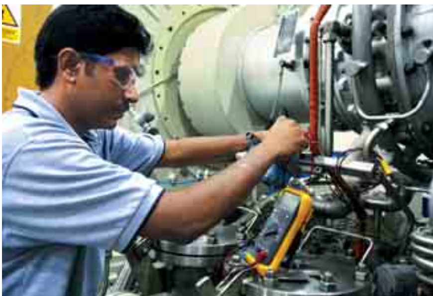
System testing on a gas turbine unit at Turboservices: Solar Turbines Integrated Service Centre.
