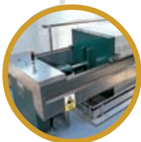
A new generation MEURA 2001 mash filter which was installed to increase the quality of wort. Periodic samples are taken to test the wort quality
