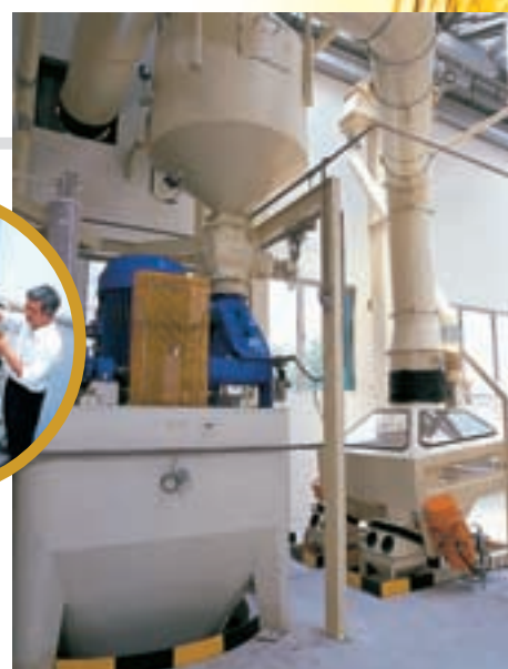
Top: Hammer mill to crush malt grain into finer form for better yield
