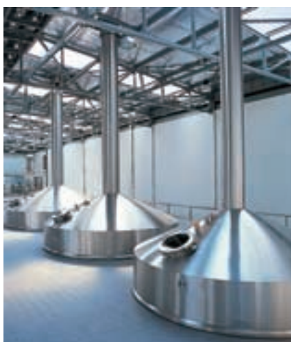
New pre-run vessel, wort kettle and whirlpool to increase the capacity in the new brewhouse
