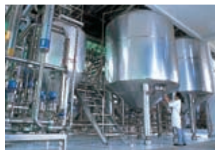
New yeast propagation plant with yeast storage tanks which are equipped with automatic valve matrix to better control yeast microbiological condition
