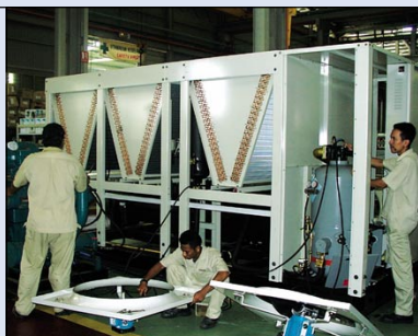
Assembly of an air-cooled vertical rotary screw flooded chiller, model ACFX at Dunham-Bush's factory in Kajang, Malaysia
