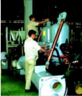
Assembly of a water-cooled vertical rotary screw flooded chiller, model WCFX at Dunham-Bush factory in Kajang, Malaysia
