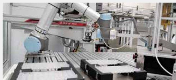
FIGURE 23: UR5 ROBOT PRECISE AND ACCURATE WORK IN FITTING TIPS INTO TRAYS
