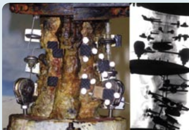
The Follower Preload Setup to simulate the physiological loading of the spine with reflective markers placed on the pars interarticularis to derive the facet kinematics in an intact and L4L5 Artificial Disc Replacement cadaver lumbar spine.
